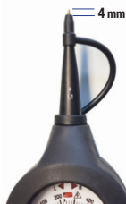
Push protective cap firmly while turning it slightly until the tip of the electrode protrudes
